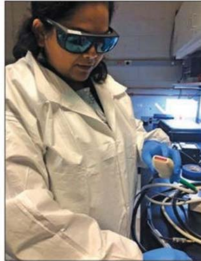
Dr. Mallidi showing an integrated probe that can obtain ultrasound and photoacoustic images simultaneously.
